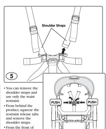
• Push to remove the shoulder straps from the waist restraint buckle slots.
